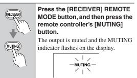
**To unmute the AV receiver,** press the remote controller's [MUTING] button again, or adjust the volume. The output is unmuted and the MUTING indicator goes off. Muting is cancelled when the AV receiver is set to Standby.
